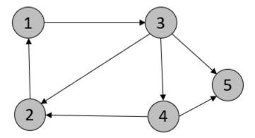
Note again that each vertex has an arrow which specifies a direction and that there are no cycles making this a directed acyclic graph. Note that there is not one specific edge (node) that can be considered the root of the graph.
